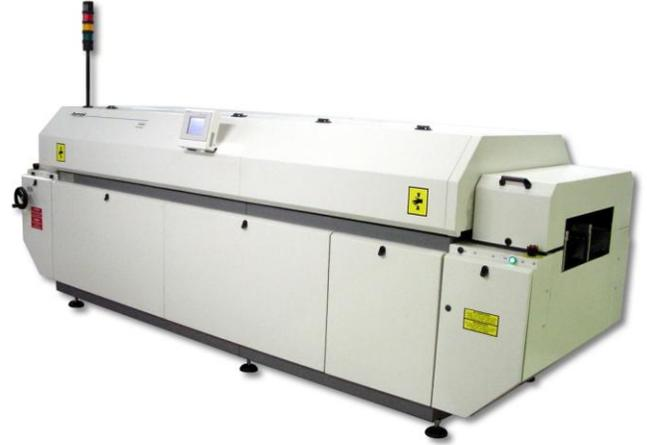
The IR/convection cure module is ideal for mid- to high-volume production. The oven features precise control of conveyor speed and internal thermal environment. Infrared panels and exclusive heat dispersion plates transfer heat by convection.
